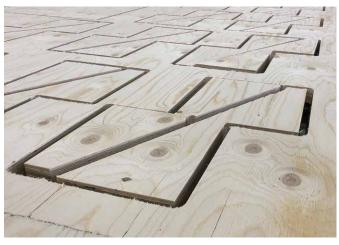
Figure 3. CNC machined Kerto LVL
